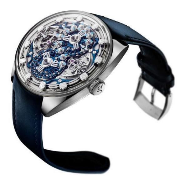
The timepiece is powered by a hand-wound manufacture calibre in 18K gold and features a variable inertia balance wheel. The main base plate is in two parts and separates energy regulation and distribution, from transmission.
